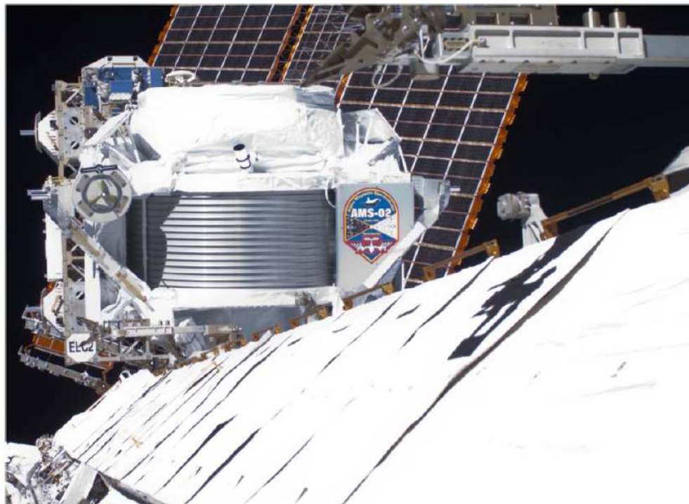
Figure 1: From its vantage point ~260 miles (~400 km) above the Earth, the Alpha Magnetic Spectrometer (AMS) collects data from primordial cosmic rays that traverse the detector.
